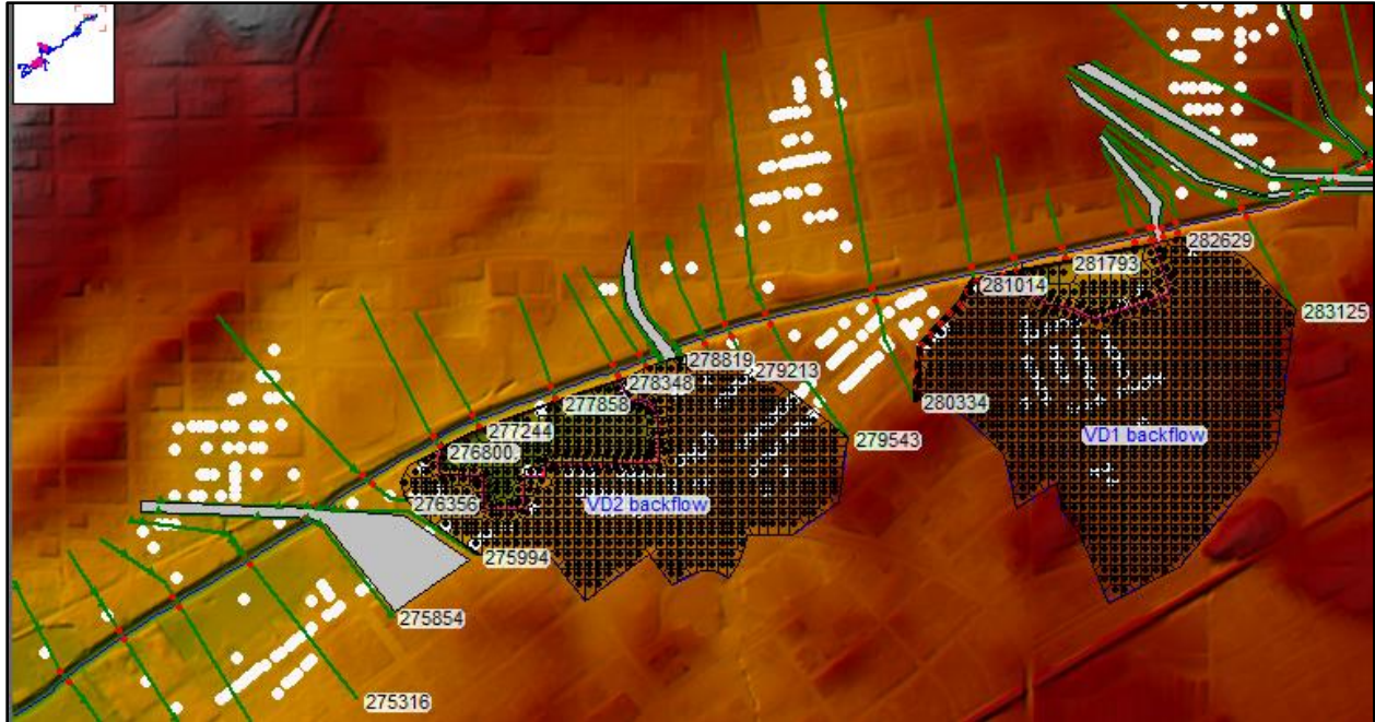
Figure 5-11: RAS schematic showing updated modeling approach in the vicinity of VD1 and VD2. Note that the 2D areas model both the ponds and their backflow areas. The pond berms are physically represented in the terrain. The same inflow weirs are utilized in the updated configuration; however, additional connections are used to properly transfer the left overbank flows from cross sections to the backflow areas, and vice-versa. The set-up of VD4 is similar. Schematic notes: north is oriented up and scale is 1:8,000.
